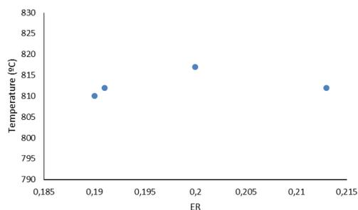
**Figure 8:** Temperature vs ER during gasifying test
