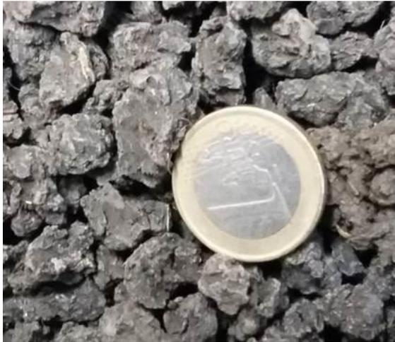
**Figure 5:** Dry sewage sludge used in the gasification test
