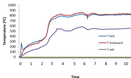
**Figure 7:** Temperature during the gasification test
