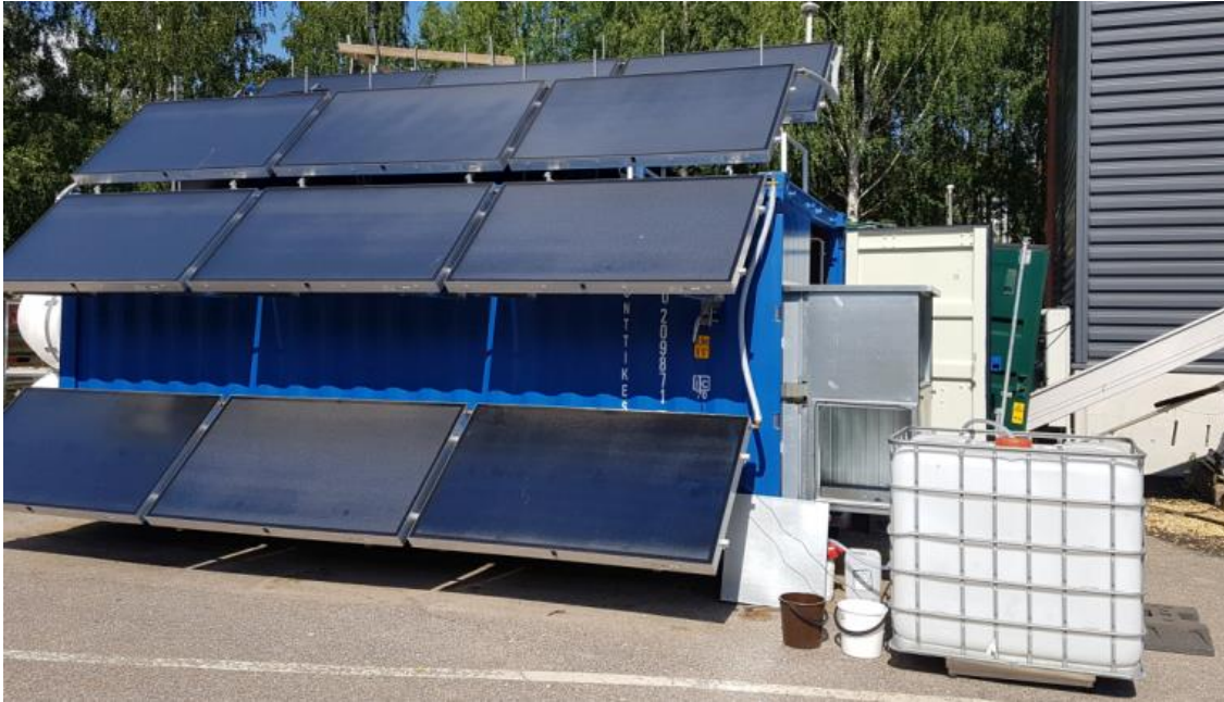
Fig. 1. Solar collectors on top of the container where the air supply unit is mounted. Source: VTT
