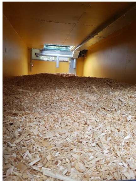
Fig. 2. Air supply unit and integrated heat pump with radiators in the container (left). The other container serves as a drying chamber (right). Biomass can be moved and circulated with a bottom agitator and chain conveyor. Source: VTT
