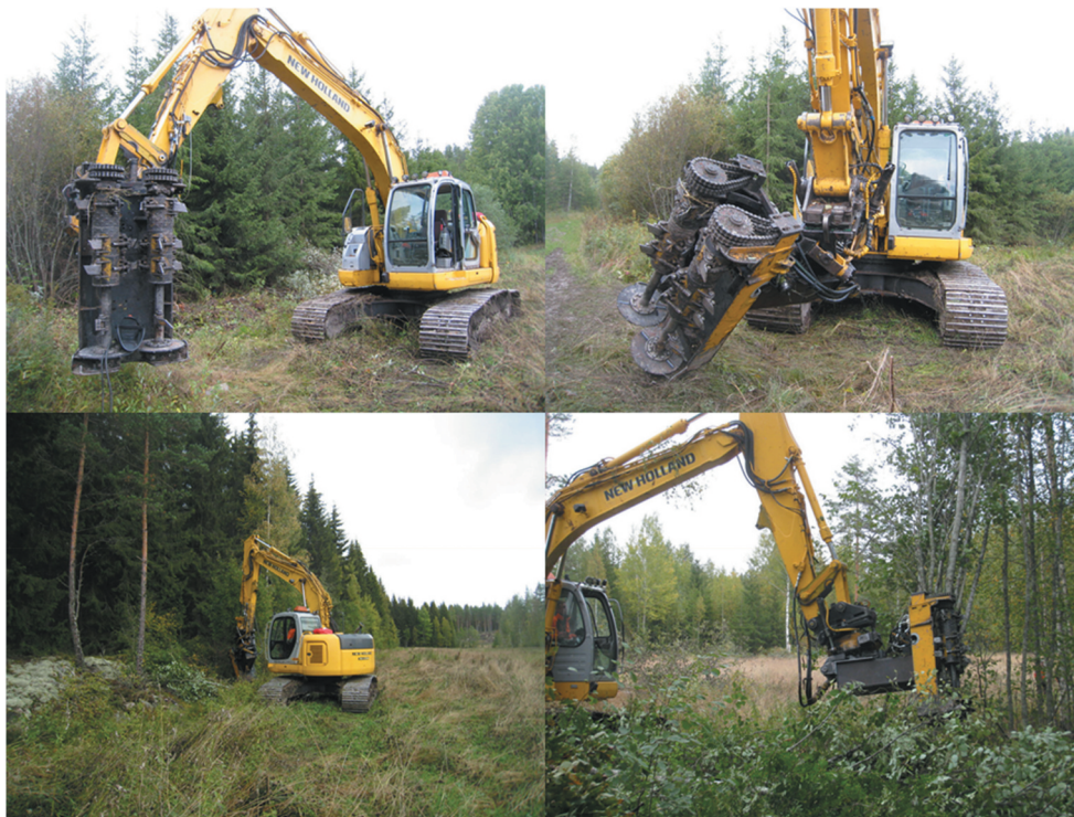
Figure 1. The integrated harvesting and clearing of brushwood were done with the Risupeto disk saw feller-buncher unit in the study. The Risupeto accumulating felling head was attached to the boom tip of the medium-sized New Holland Kobelco E 200 SR crawler excavator.
