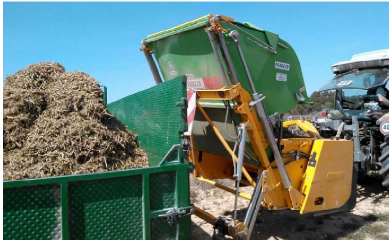
Figure 6: The Cobra Colina (PERUZZO) unloads vineyards pruning chips to a trailer (Source: CIRCE).
