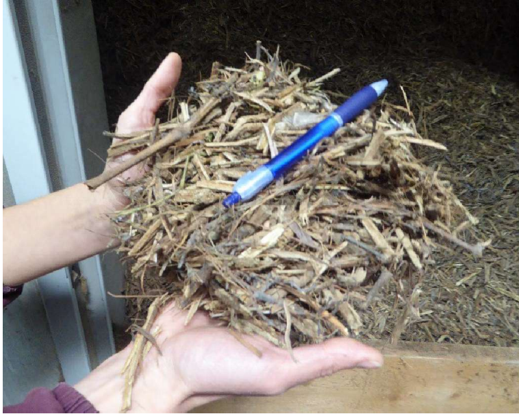
Figure 8: The inhomogeneous biomass (hog fuel) from vineyard prunings consumed at Vilafranca district heating (Source: CIRCE).
