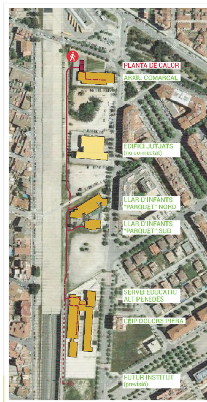
Figure 10: Sketch of the district heating fed with vineyard prunings (source Vineyards4Heat)
