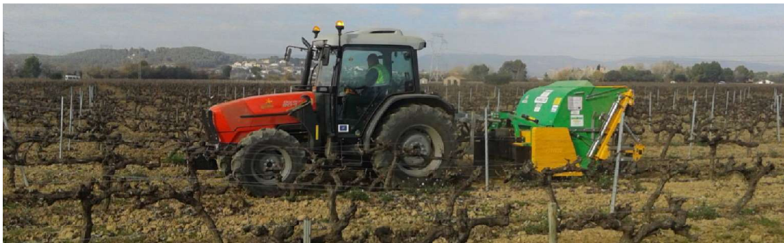
Figure 5: Harvesting + pre-treatment process using the Cobra Collina B1400 (Source: Vineyards4heat).
